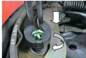
1. hold the handle, clip groove the front ditch and rotation the tool
