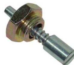
KA-2877 Injection Pump Lock Pin-Late Model ■ Locks diesel pump cam to maintain timing during pump installation ■ Mercedes Benz: 601, 602, 603, 604, 605, 606, and 617.
